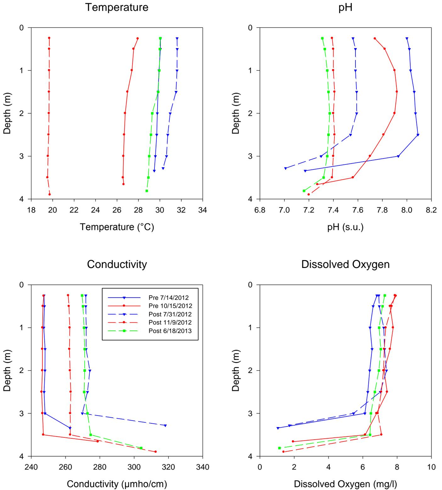
Figure 3-11. Pre- and Post-Treatment Vertical Field Profiles Collected in the Southwest Lobe.
