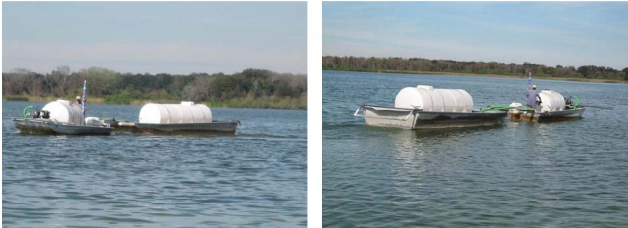
Figure 2-5. Application Boat and Tanker Barge Used for Alum Application in Lake Jessamine.
