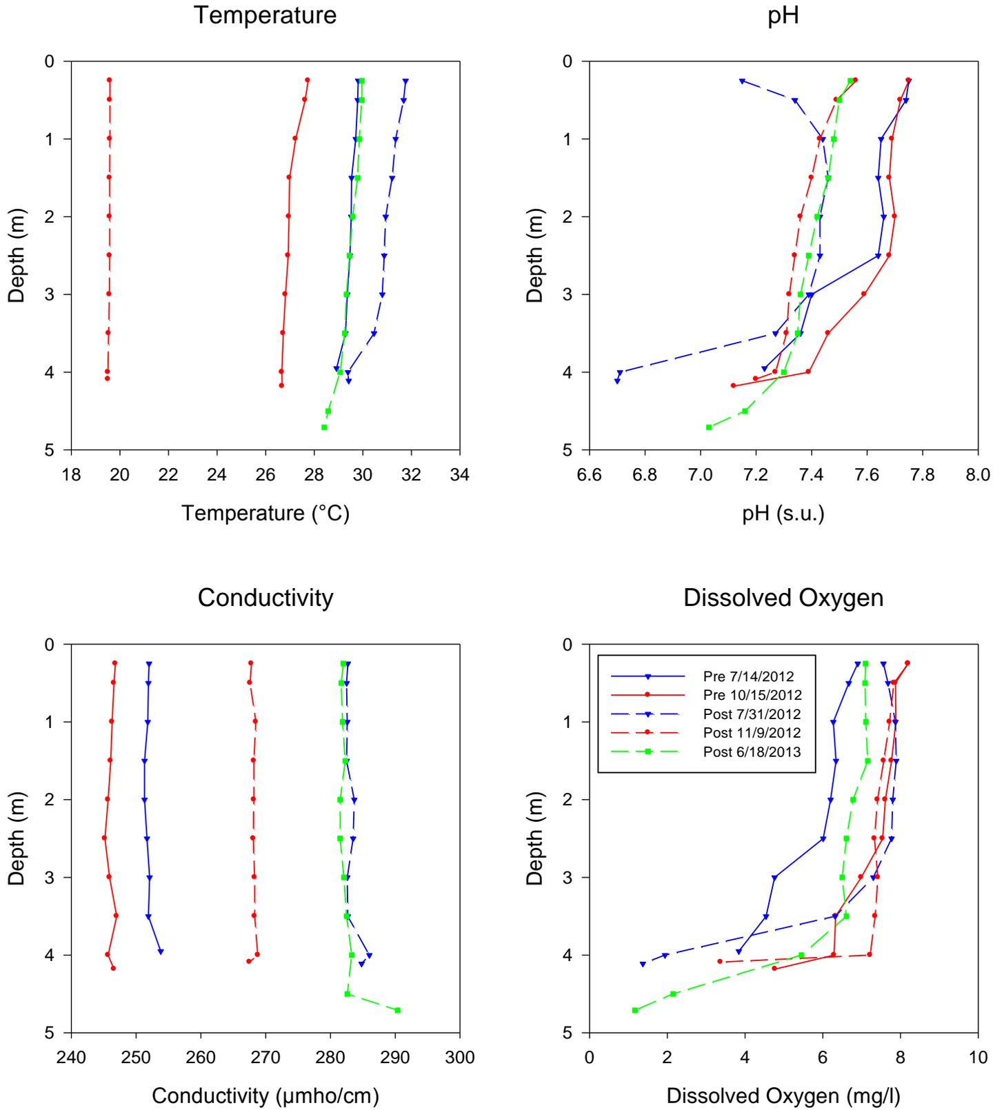
Figure 3-9. Pre- and Post-Treatment Vertical Field Profiles Collected in the Northeast Lobe.
