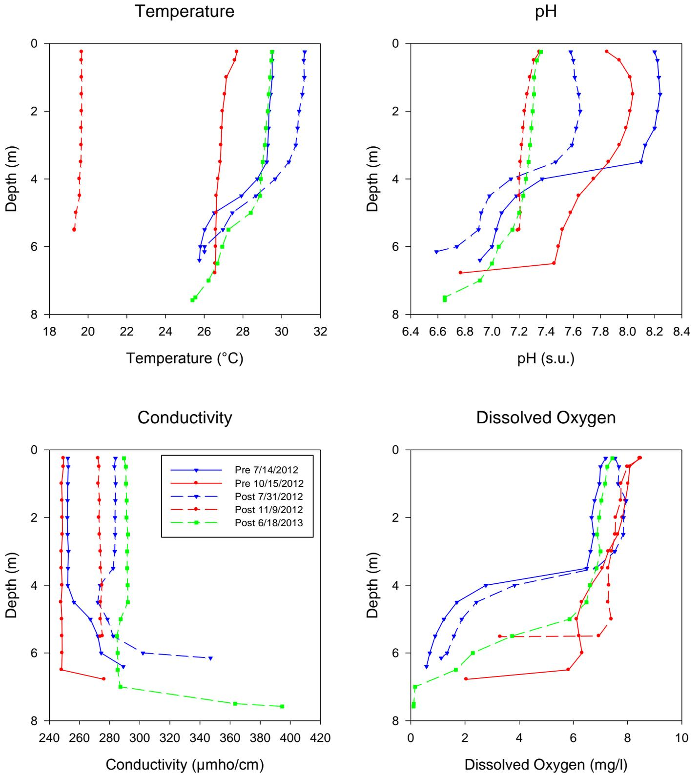
Figure 3-10. Pre- and Post-Treatment Vertical Field Profiles Collected in the Middle Lobe.
